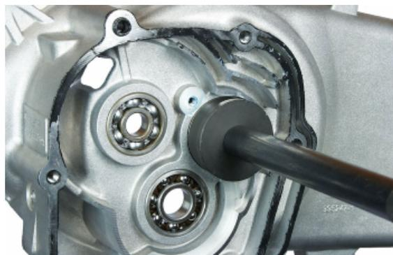
**Fitting the Intermediate gear bearing**
