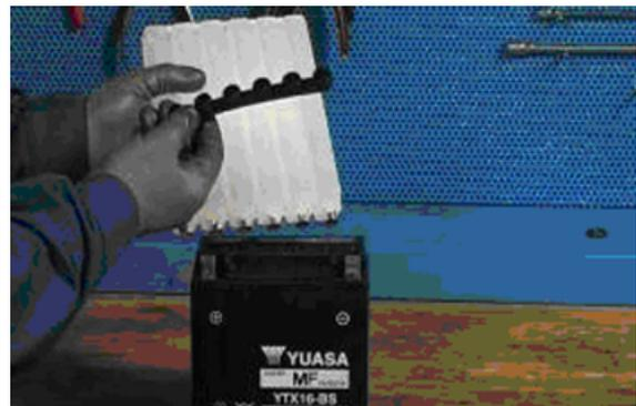
**3) Procedure for filling the battery with acid.**
