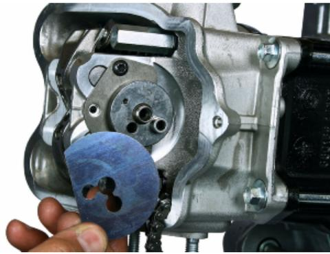
After removing the head the camshaft control components can be removed:
