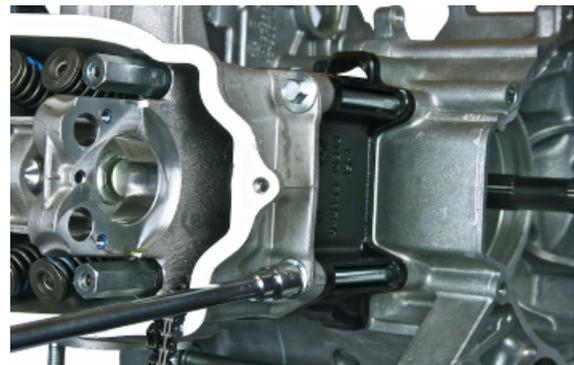
Fit the pins and rocking levers.
