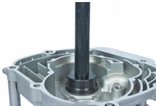
**Fitting the Wheel axle bearing**
