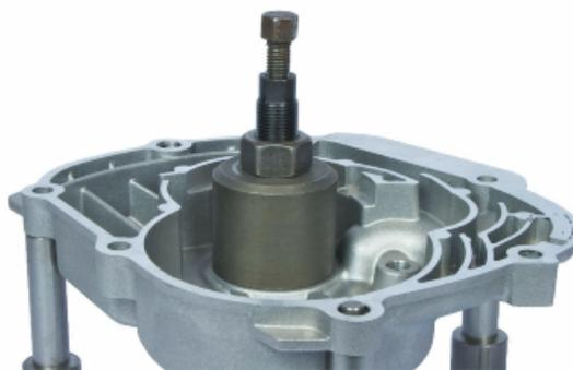
**FITTING****Fitting the Intermediate gear bearing**
