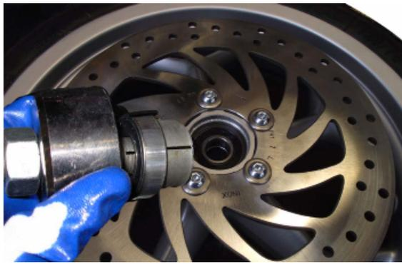
**Specific tooling****020151Y Air heater****001467Y003 Nut****001467Y009 Bell for OD 42-mm bearings****001467Y019 Extraction pliers for  $\varnothing$  18 mm bearings**
