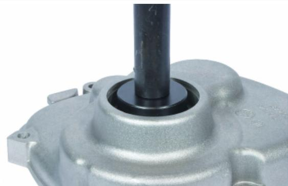
**Removing the intermediate gear bearing**
