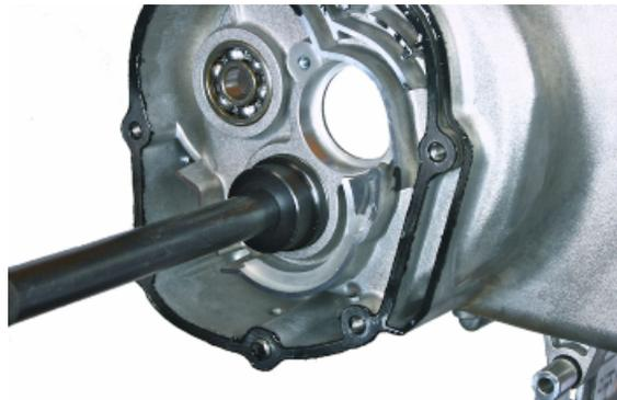
**Fitting the Clutch shaft bearing**
